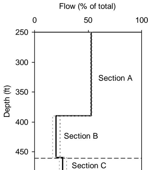
Figure 3. Benevides-Duval County CD Well 1 discharge profile showing the percentage of total well production originating from the tested screen sections (black line). Values for screen section C are based on the system flow meter. Short dashed lines represent flow percentage uncertainty. Horizontal long dashed line represents the pump setting depth (462 ft).
