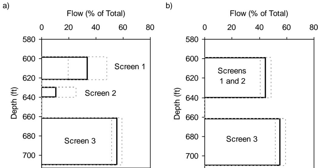
Figure 1. Riviera Water Supply Well 2 discharge profiles expressed as a percentage of total discharge for a) individual screens and b) combined screens 1 and 2. The pump is set at the 265 ft depth.
